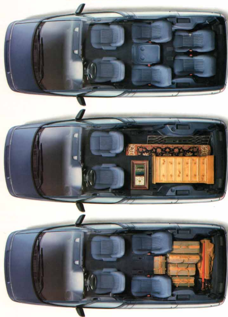
A number of flexible seating configurations provide a wide variety of easily created seating and cargo hauling options. Besides being removable, the last two rows of seats can also be folded down to become tables with handy cup holders.
