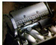
(Top) The 160-horsepower, 2.3-liter Quad 4 engine with multiport fuel injection—standard on the Achieva SL. (Bottom) The 120-horsepower, 2.3-liter Quad Overhead Cam with multiport fuel injection—standard on the Achieva S.
