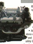
The 3300 multipoint injected V6 engine and a four-speed automatic overdrive transmission are both standard on the Cutlass Cruiser SL.
